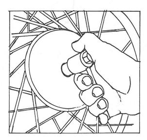
REMOVES SPECIAL LOCKING LUG NUTS WITHOUT DAMAGE TO THE LOCK ON WHEEL/STUD.
